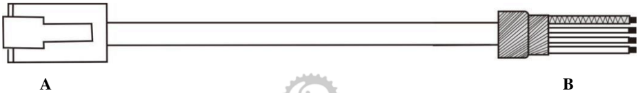
Pic 4.10 The Communication Cable Of Servo Drive With PLC
